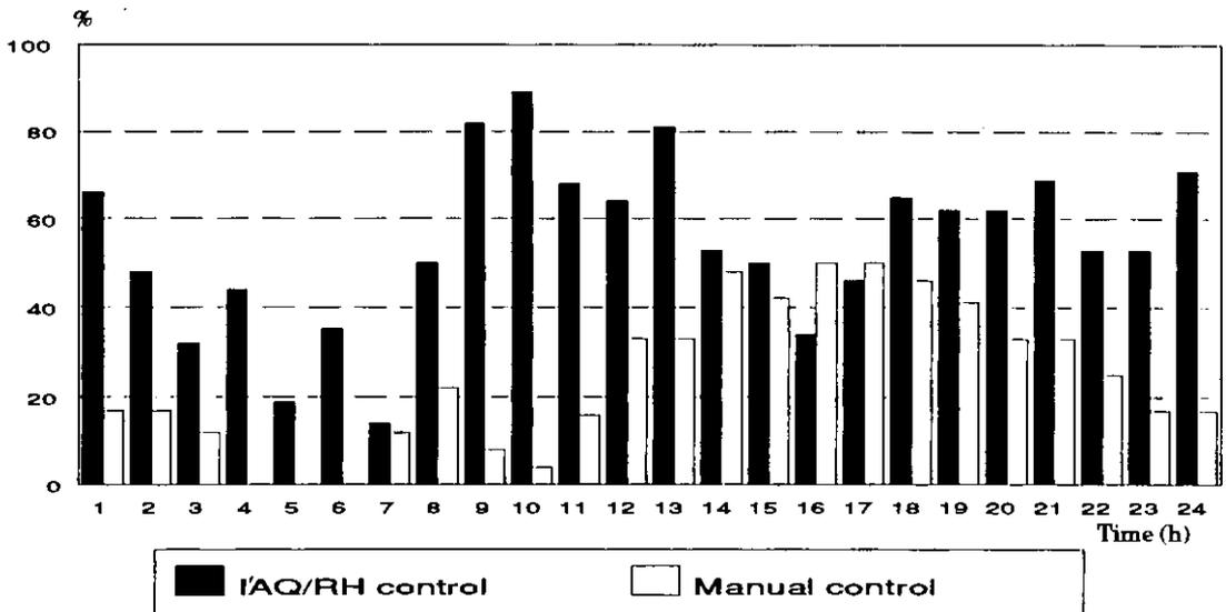
**Figure 7.12. Percentage of time of fan operation at high speed as a function of time of the day**
