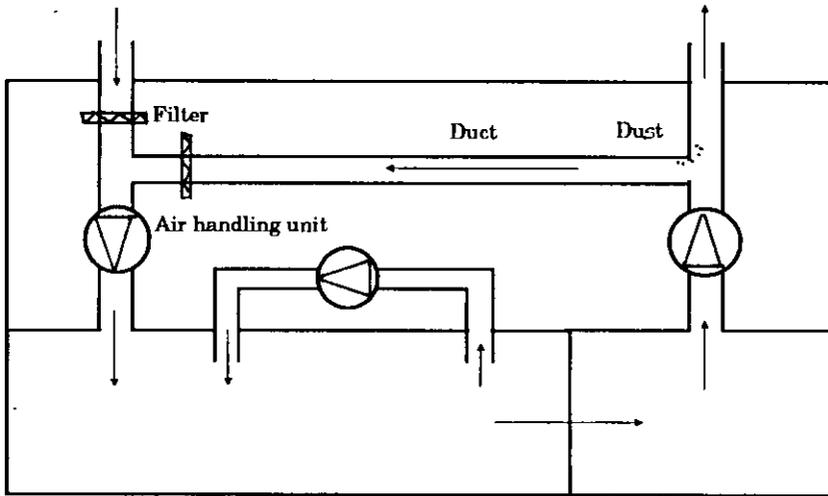
Figure 3.2 Pollutant sources in a ventilating system
