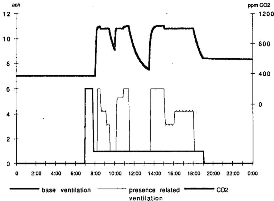
*Figure 5.11. Ventilation operation with variable air flow*
