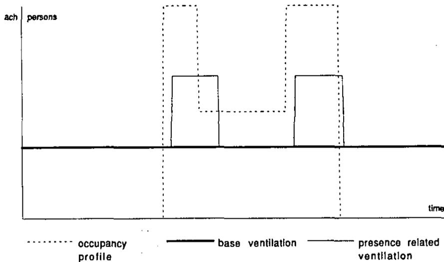
*Figure 5.1. Combination of base ventilation rate and occupancy ventilation rate*
