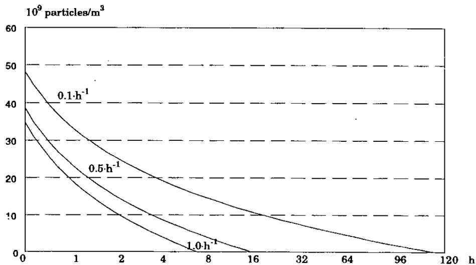
Figure 3.1 Dilution of tobacco smoke by ventilation in a room ( $50 \text{ m}^3$ ,  $0.5 \text{ h}^{-1}$ ).
