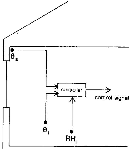
The surface temperature is directly measured at the critical/coldest spot of the wall (see [4]).
