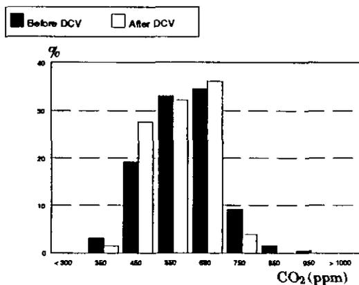
Percentage of time for given CO<sub>2</sub> concentration. Average after DCV 558 ppm. Average before DCV 584 ppm.
