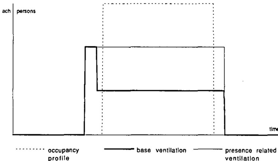
Figure 5.6. Constant and known pollutant source strength with constant system operation during the service time of the building
