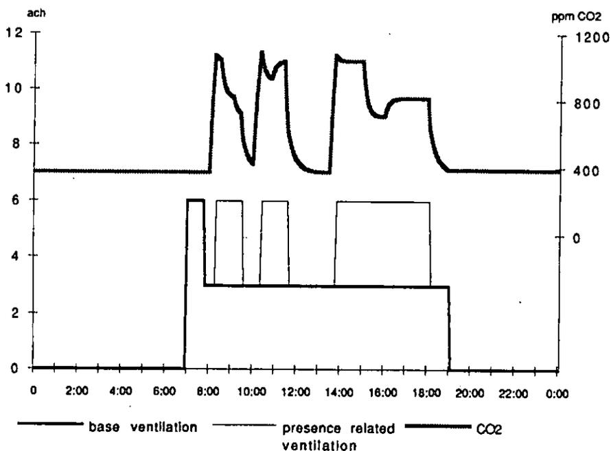
Figure 5.10. Ventilation operation with two-speed fan
