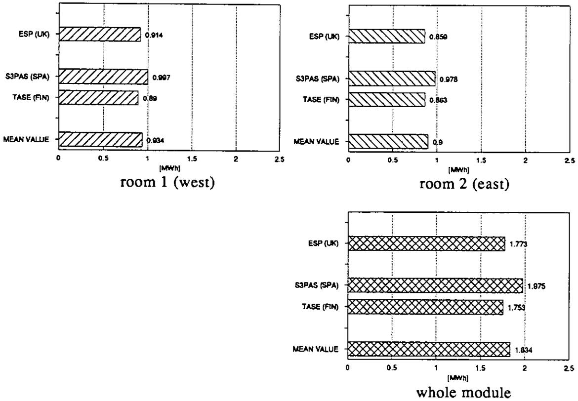
Figure 14.2a Annual heat losses through windows in case 2a.
