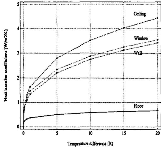
Figure 2. Convective heat transfer coefficients for interior surfaces.
