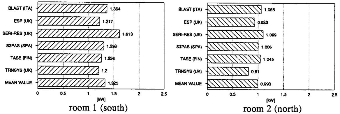
Figure 10.1a Annual peak cooling loads for both rooms in case 1a.
