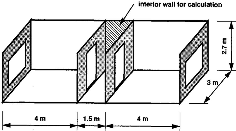
Figure 1. The module of the commercial building.
