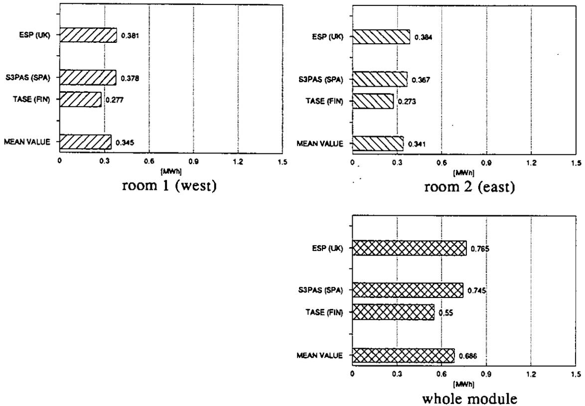
Figure 13.2b Annual heat losses through exterior walls in case 2b.
