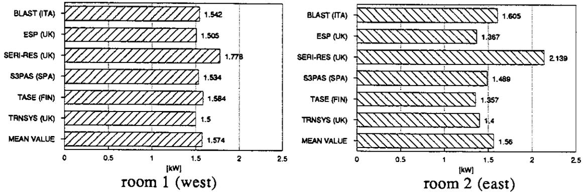
Figure 10.2a Annual peak cooling loads for both rooms in case 2a.
