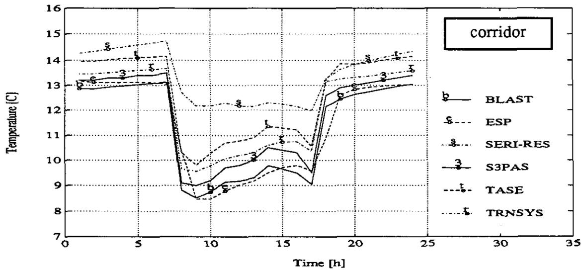
Figure 16.3b Room air temperatures for both rooms and corridor on January 4th in case 3b.
