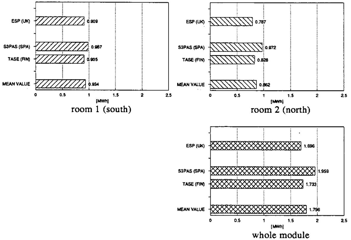
Figure 14.1a Annual heat losses through windows in case 1a.
