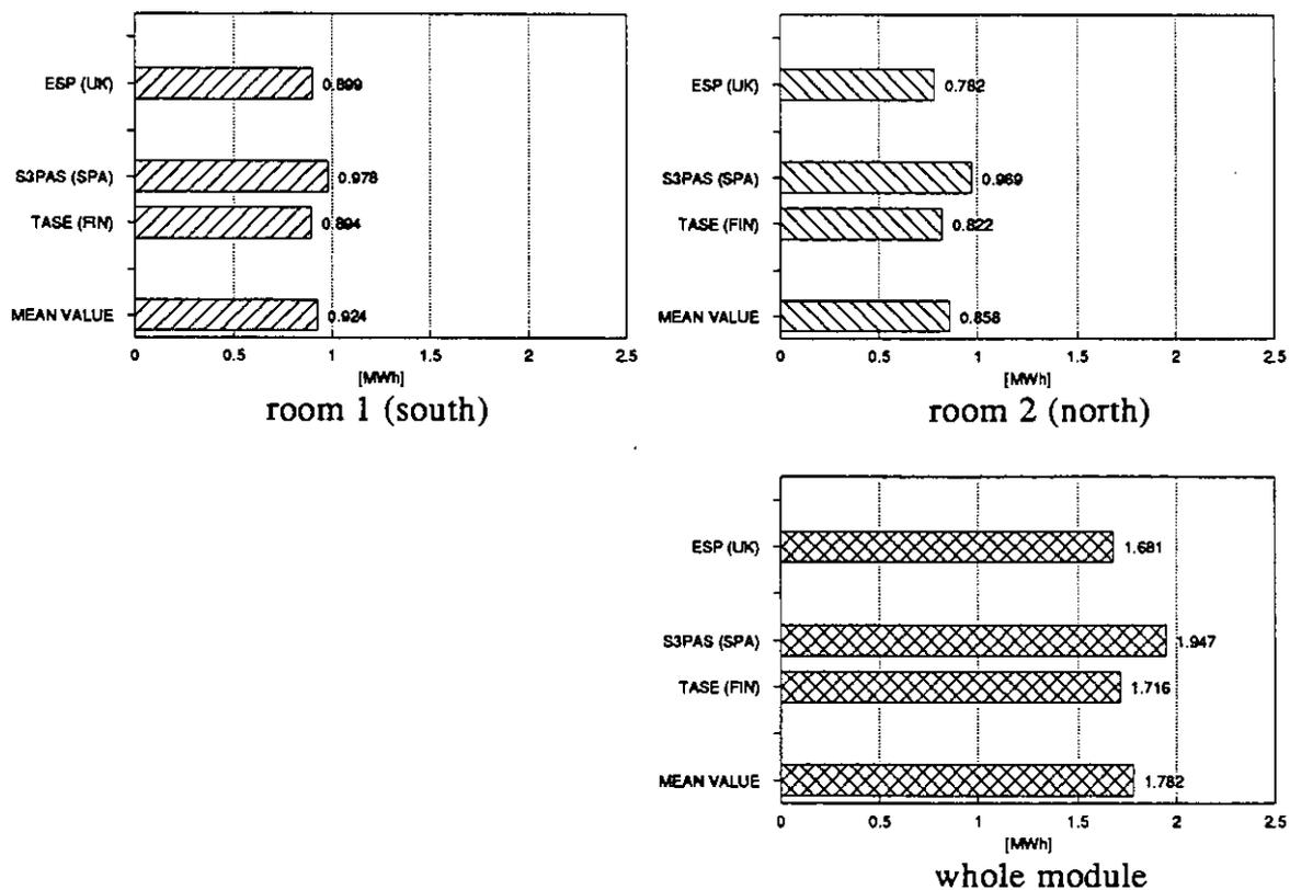
Figure 14.3a Annual heat losses through windows in case 3a.
