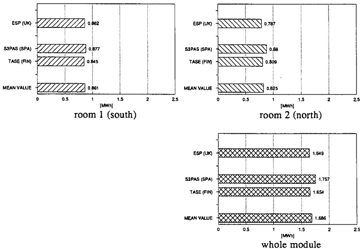
Figure 14.3b Annual heat losses through windows in case 3b.
