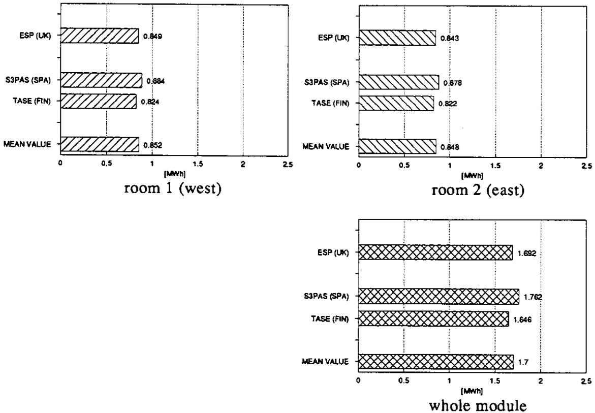
Figure 14.2b Annual heat losses through windows in case 2b.
