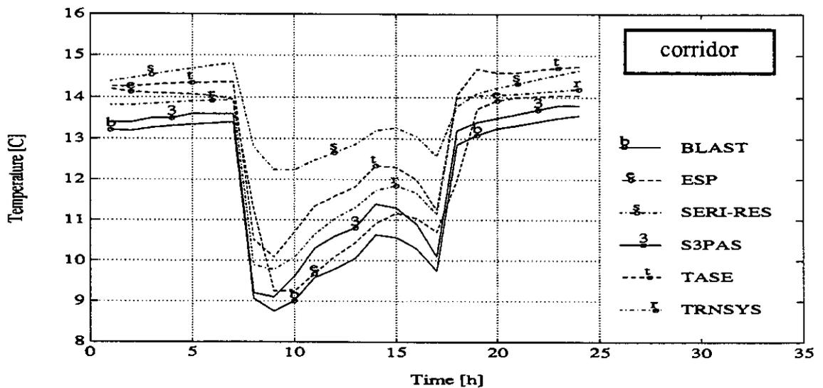
Figure 16.3a Room air temperatures for both rooms and corridor on January 4th in case 3a.
