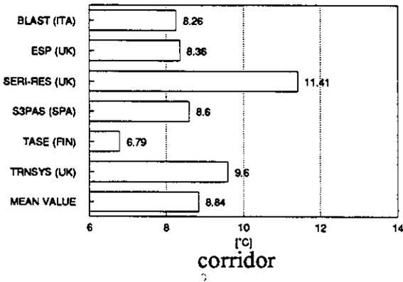
Figure 12.3b Minimum annual air temperature for corridor in case 3b.
