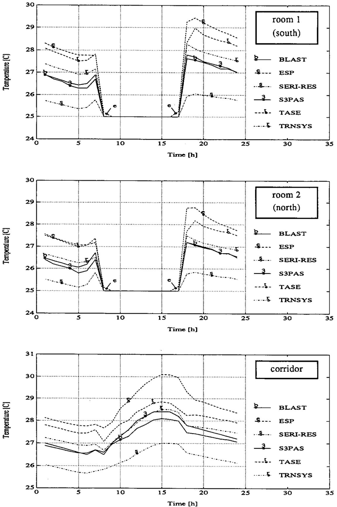
Figure 17.3a Room air temperatures for both rooms and corridor on July 27th in case 3a.
