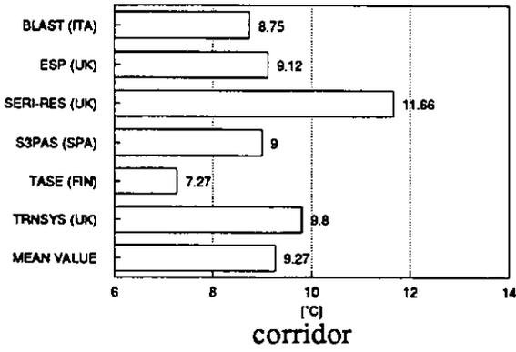
Figure 12.3a Minimum annual air temperature for corridor in case 3a.
