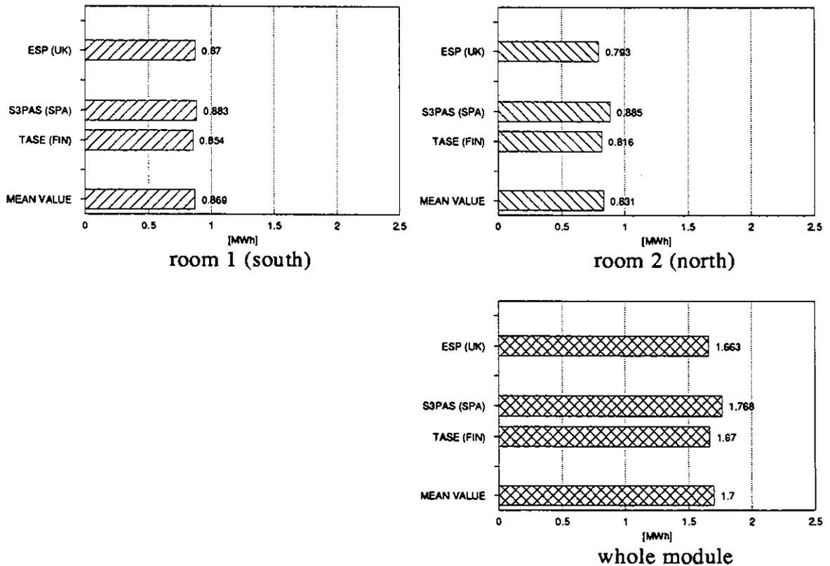
Figure 14.1b Annual heat losses through windows in case 1b.
