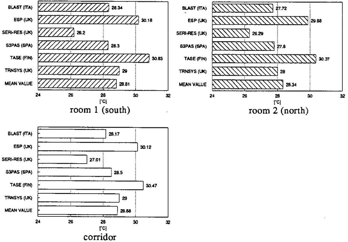
Figure 11.3a Maximum annual air temperatures for each space in case 3a.
