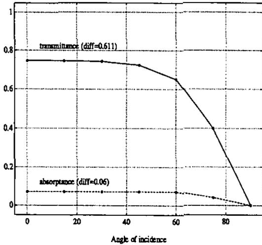
Figure 1. Transmittance and absorptance of window.
