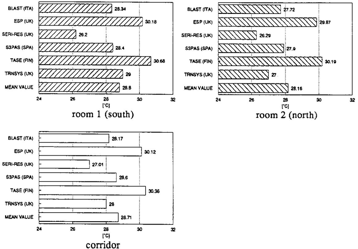
Figure 11.3b Maximum annual air temperatures for each space in case 3b.
