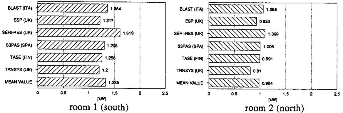
Figure 10.3a Annual peak cooling loads for both rooms in case 3a.
