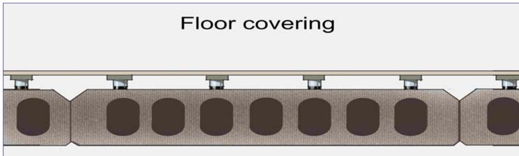
Figure 3-20 Principle of a hollow deck with cavities for air circulation
