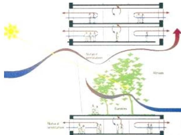
The atrium works as a chimney for the ventilation air. The winter-gardens also work as a thermal buffer during the winter and summer season. In winter it is used to preheat the natural ventilation, while in summer it is used to cool down the external air by 0.5 and 1°C through evaporative cooling. [Need permission](#)
