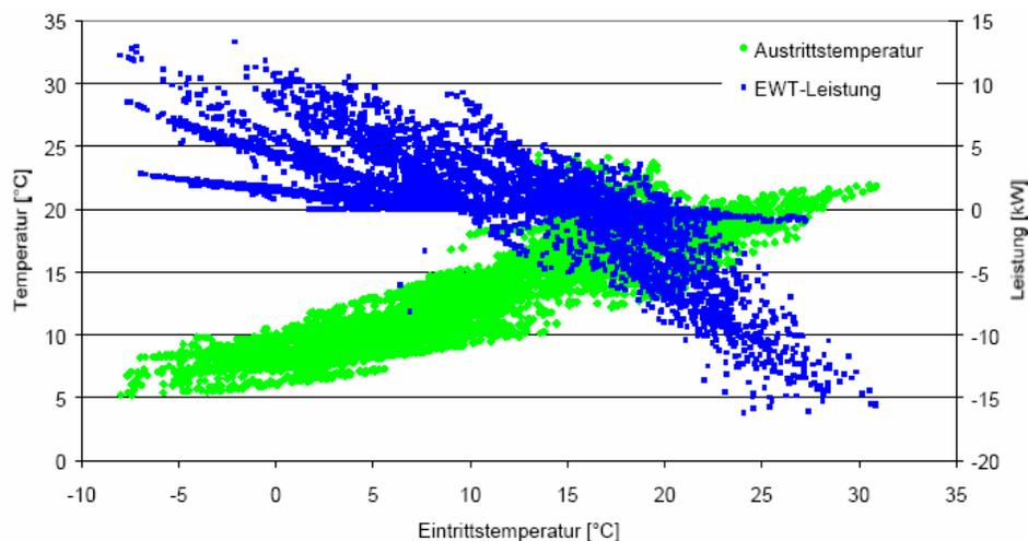
The underground heat exchanger performance and the outlet temperatures as a function of the inlet temperature. (*Eintrittstemperatur* = inlet temperature and *Leistung* = yield of the underground heat exchanger).
