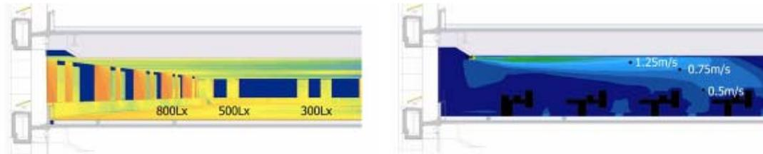
For taking in a skylight as much as possible while blocking the direct solar radiation effectively, the energy of illumination is reduced. First, a ceiling near the window is bent up to maximize a window height up to the lower part of the 'Eco-Frame'. Second, window shades that climb up from the bottom are adopted, and these techniques are automatically controlled according to an annual schedule based on sun position and presence of the direct solar radiation measured by lighting sensors.
