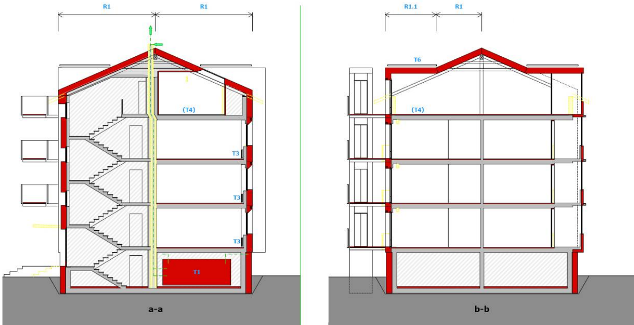
Figure 10: Cross-section with new building envelope as well as direct heated and indirect heated rooms (hatching)
