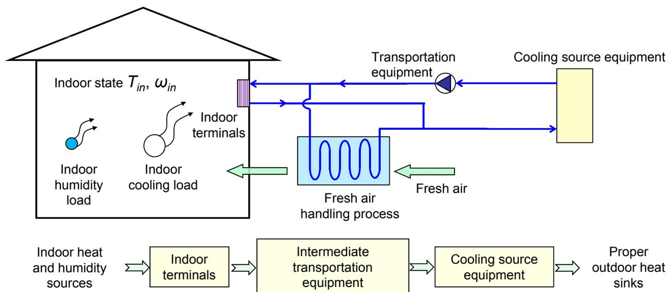
The main processes in an active air conditioning system. This contains a series of processes, including collection, transport and cooling source equipment.
