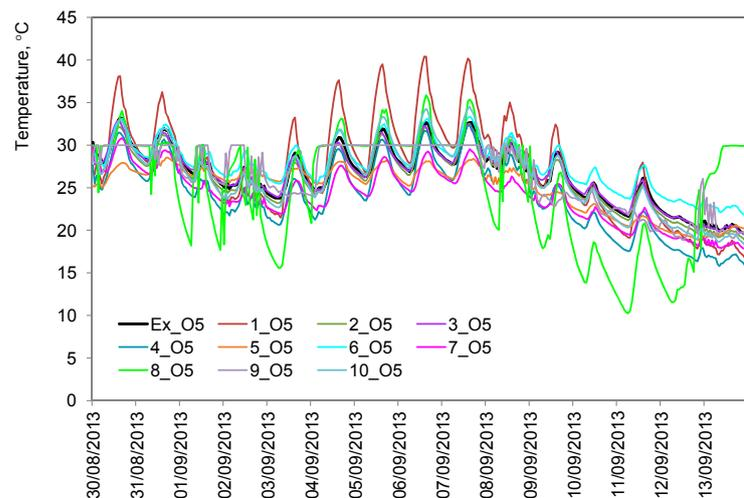
A living room at the Twin Houses, a Fraunhofer IBP experimental facility (left). Test house 05 ROLBS experimental data (right) for living room temperatures (Ex\_O5), with simulated results from 10 programs (1\_O5 to 10\_O5). The timeline comparisons show some simulated results are clearly erroneous, but others give good levels of agreement overall. No simulation program predicted the temperature in every room and in every period to within 1°C, although two came close.
